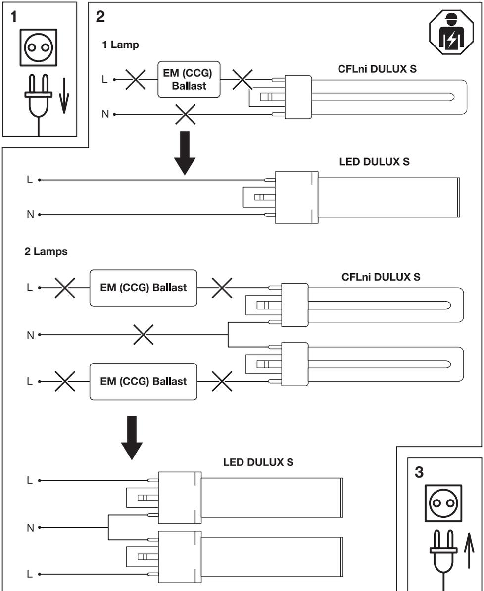
The fixtures electrical circuit/wiring has been modified and can now no longer operate traditional DULUX lamps. Use only with approved LEDVANCE DULUX LED. Please mark luminaire with a warning sticker included in the LED tube packaging. <sup>4)</sup>
