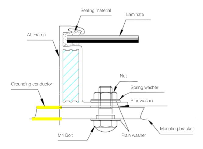
When grounding, each module can be grounded directly or in series or in parallel. If you choose the latter two options, it is recommended that the maximum number of modules connected in parallel should not exceed four, and in series should not exceed eight.
