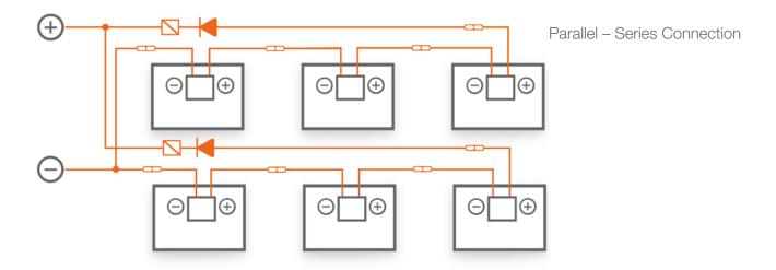
Before the commissioning and operation of the power station, check the electrical connection of modules and strings, making sure all connection polarity is correct and the open circuit voltage meets the requirements of the acceptance criteria.
