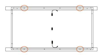
Installation with bolts into 4 outer holes (Beam Parallel to long sides)
