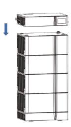
Finally, install the high voltage box to the top layer of the battery module
