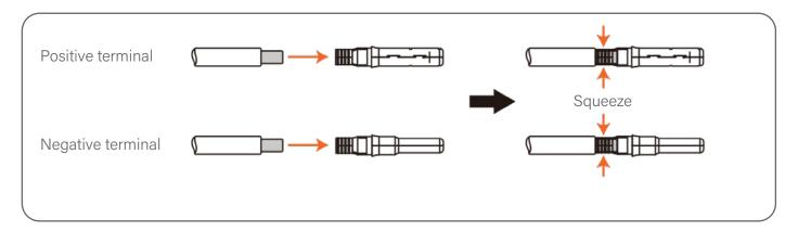
5. Insert the crimped DC cable into the DC terminal firmly, then insert the waterproof rubber ring into the DC terminal and tighten the nut.
