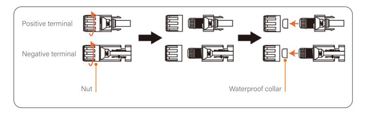
3. Pass the stripped DC cable through the nut and waterproof rubber ring.
