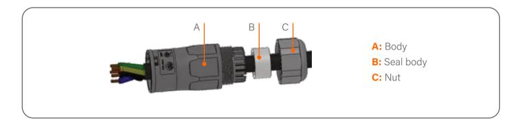
3. Crimp wires, screw torque 0.8Nm±0.1Nm.
