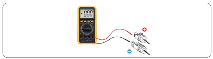
Step 2: Measure AC voltage and frequency and ensure they are within local standard.
