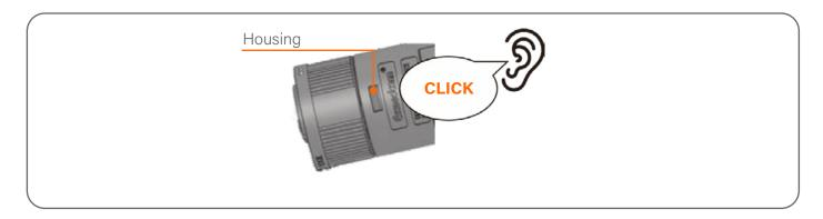
5. Insert seal body and claw into the body, and then tighten the nut with torque 2.5Nm±0.5Nm.
