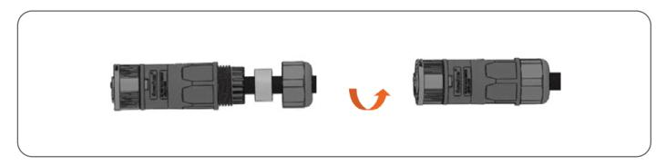
6. Push the AC backup connector into the AC backup port on the inverter and rotate the rotatory ring on the AC backup connector to the direction as marked "LOCK" on the connector (hold the body while rotating the ring).
