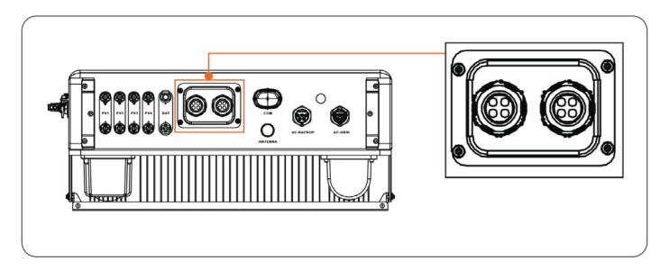
Inverter in the package is with a protective cover assembled to protect the communication ports.
