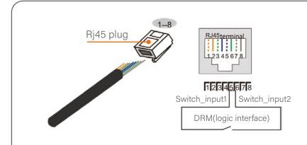
Correspondence between the cables and the stitches of plug, pin5 and pin6 of RJ45 terminal is used for the logic interface, other pins are reserved.
