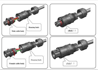
5. Push the sealing body and sealing craw into the housing body, and then tighten the end locker, torque 4.0±0.5 N·m.
