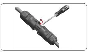
8. If the connector to be disassembly for rewire, please according to the following steps: Loosen tail parts (End Locker); Use a suitable flat screwdriver to press the elastic
