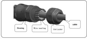
6. When mating connectors, align mate-locker on the male connector with grooves on the female connector, and insert gradually. Connected in place, there will be a sound of "click".
